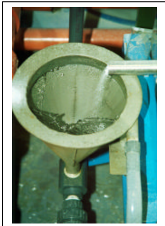
Polymer feed into the Washdown Funnel and being drawn through the Jet Eductor
